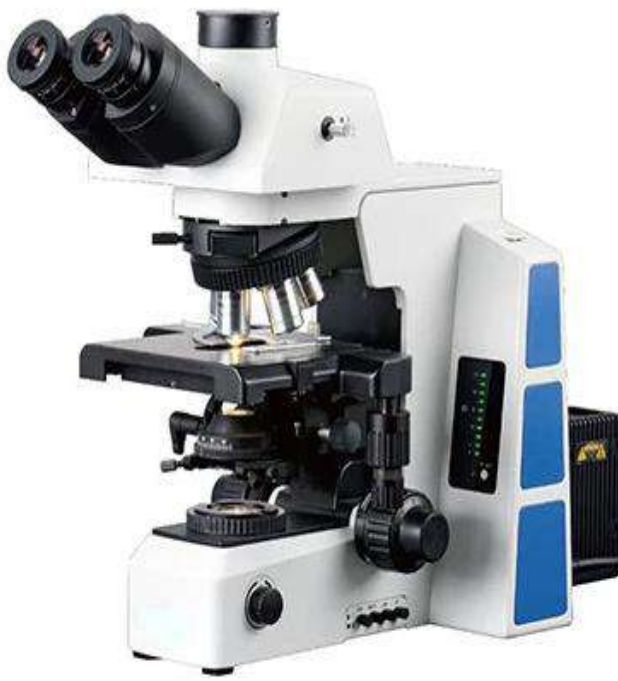
SLV-61i Research Scientific Laboratory Microscope, Semi-APO, Upgrade BF+DF+PL+PH+FL+DIC
